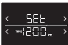
After connecting your appliance to the power for the first time, or after an extended power outage, 12:00 will flash on display.
