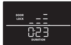
Briefly press the **Self Clean** key and touch **<** or **>** to set the desired cleaning intensity. Confirm the settings by pressing on the **OK** symbol. Lock and program duration will appear on display (the door will be locked). The default cleaning duration is 3 hours.
