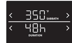
Baking during **Sabbath Mode**. Set the baking temperature and time. The default temperature of 350 °F is displayed at the top of the display unit. You may adjust the temperature in the range from 175 °F to the maximum possible setting of 425 °F. The default time of 48 hours is indicated at the bottom of the display unit. You can set it in the range from 1 hour to 74 hours.
