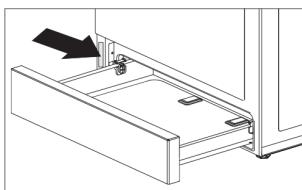
The rating plate indicating the basic information about the appliance is located on the oven frame and it is visible when the oven door is opened.
