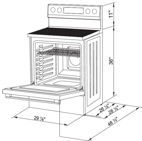
See illustrations for all rough-in and spacing dimensions. The appliance may be placed with 0" clearance (flush) at the back walls and side walls of the cabinets.
