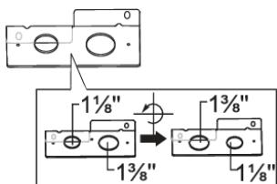
Remove the conduit connection plate by removing two screws and rotating it, as shown below. The conduit hole (1 1/8") must be used. Tighten both screws back.
