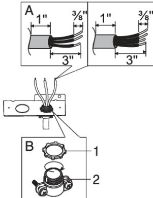
Prepare the conduit cord (insulation stripped) as shown in A.
