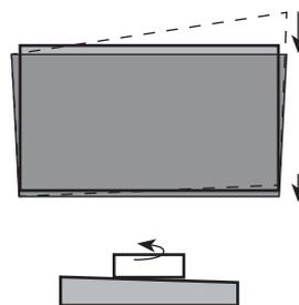
3. Repeat the steps above until the top of the image is parallel with the screen.
