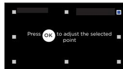
2. Adjust the position of the point by pressing the UP/DOWN/LEFT/RIGHT buttons, then press the Back button to view and select other points. Your changes will apply automatically.
