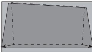
NOTE: Make sure the bottom of the image always stays parallel with the screen. If not, rotate the Laser Cinema following previous instructions.
