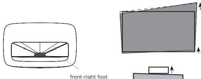
2. Now, rotate the Laser Cinema counterclockwise so that the bottom of the image is parallel with the screen.
