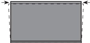
If the top of the image is narrower than the screen, then use the wrench to rotate the left- and right-back feet of the Laser Cinema clockwise, until the left and right borders of the image are parallel with the screen borders.
