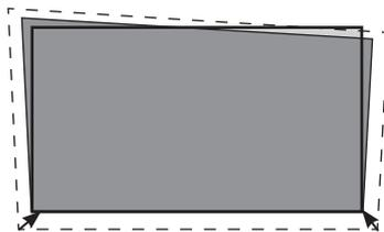
If the bottom of the image is narrower than the screen, then move the Laser Cinema farther from the screen.
