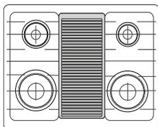
The reversible cast iron griddle can only be used over the center burners of the rangetop. Make sure the grid is correctly placed before you turn on the burner.
