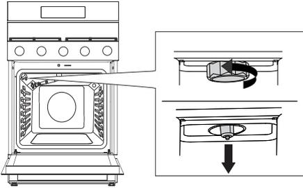
Unscrew and remove the cover in counter-clockwise direction and pull out the bulb.
