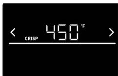
The Crisp mode can be activated and deactivated with a long press on **Crisp Mode**. In the crisping process, it's possible to start, when the set temperature of the oven is reached. The maximum duration of Crisp mode operation is 5 minutes.
