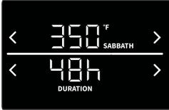
Baking during **Sabbath Mode**. Set the baking temperature and time. The default temperature of 350 °F is displayed at the top of the display unit. You may adjust the temperature in the range from 175 °F to the maximum possible setting of 425 °F. The default time of 48 hours is indicated at the bottom of the display unit. You can set it in the range from 1 hour to 74 hours.
