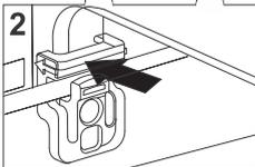
2 Simultaneously push the two spacers, one on either side, back in the direction of the arrow.
