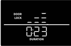
Briefly press the **Self Clean** key and touch < or > to set the desired cleaning intensity. Confirm the settings by pressing on the
