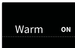
This mode allows you to keep cooked food warm. The temperature for this program can be set from 140 °F to 210 °F, and the Cooking Time can be set from 0 minutes to 3 hours. Recommended Cooking Time is 30 minutes.
