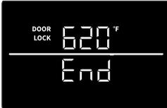
When the temperature drops to below 400 °F, the appliances will unlock and go to a stand-by state. Once the oven cavity has fully cooled down, wipe it with soap and a soft cloth to remove any residue (e.g. ashes).
