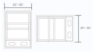
The window installation kit allows you to install the air conditioner in most vertical sliding windows 25" to 50" wide, or horizontal-sliding windows from 18" to 50" high.
