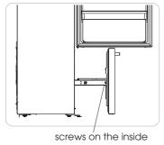
5. Pull out the freezer door and lift it up in the direction of the arrow.
