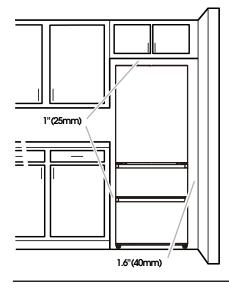
To ensure proper ventilation for your refrigerator, allow for a 1"(25mm) space on each side and at the top. Allow at least 2.0"(51mm) between back of cabinet and the wall. If your refrigerator has an ice maker, allow extra space at the back for the water line connections.
