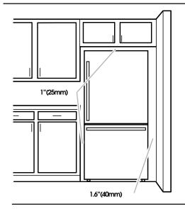
To ensure proper ventilation for your refrigerator, allow for a 1"(25mm) space on each side and at the top. Allow at least 2.0"(51mm) between back of cabinet and the wall. If your refrigerator has an ice maker, allow extra space at the back for the water line connections.
