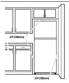
To ensure proper ventilation for your refrigerator, allow for a 3.9"(100mm) space on each side and at the top. Allow at least 3.0"(76mm) between back of cabinet and the wall. If your refrigerator has an ice maker, allow extra space at the back for the water line connections.
